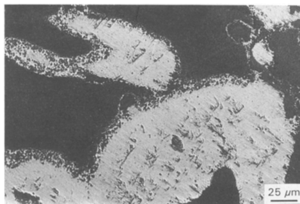
Figure 2 Optical micrograph of a titanium particle, showing a TiC layer, produced by solid-state diffusion.
